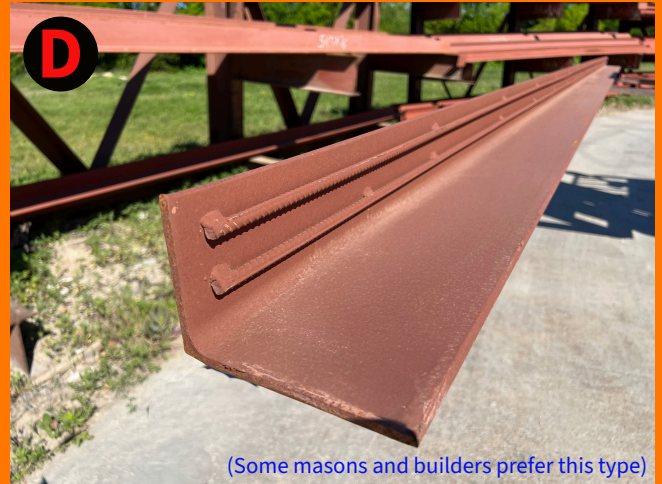
D (Some masons and builders prefer this type) 6x4x5/16" primed lintel w/ (2) #3 rebar welded to the 4" leg
