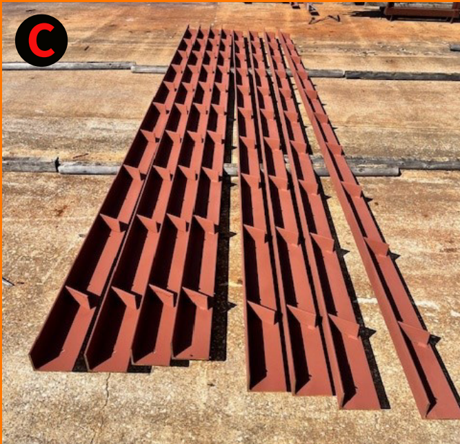
C 6x4x5/16" primed lintel w/ stops pitched right
