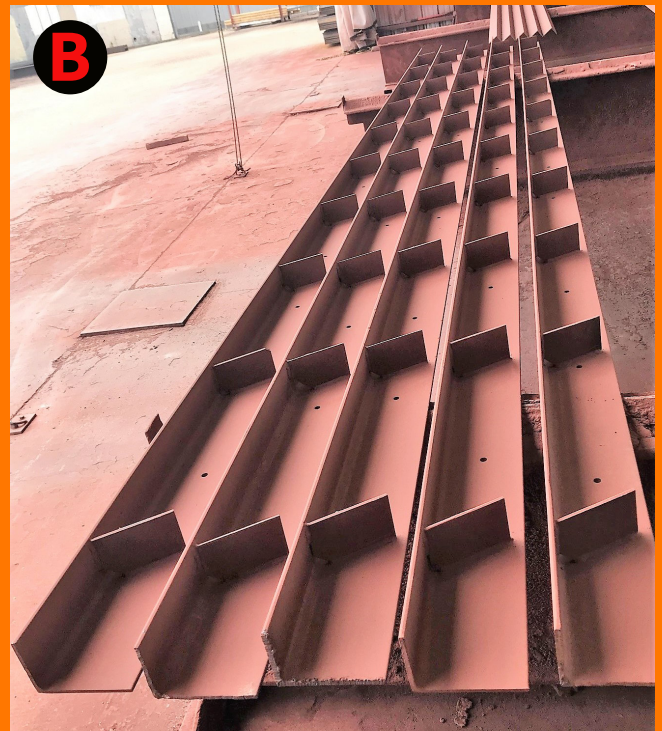
B 6x4x5/16" primed lintel w/ stops pitched left
